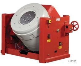
V9x Shakers are trunnion-mounted, either free-standing or as part of shaker/slip table combos. Trunnion mounting allows the shaker to be used in either the horizontal or vertical axis. The trunnions are supported by LDS' Lin-E-Air suspension system, which enables low frequency operation at full displacement.
